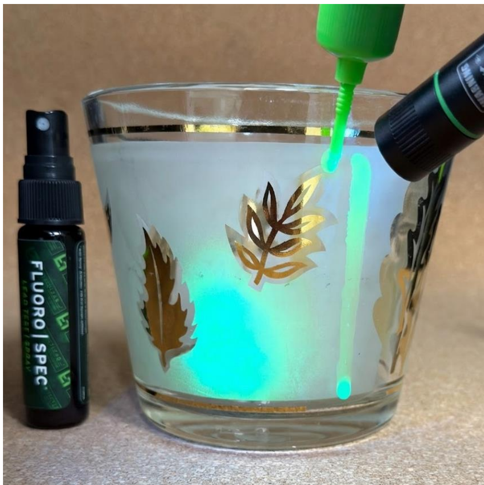
A FluoroSpec test on a drinking glass under 365-nanometre UV light: the painted decoration fluoresces bright green where lead is present. Photo courtesy of detectlead.com .
