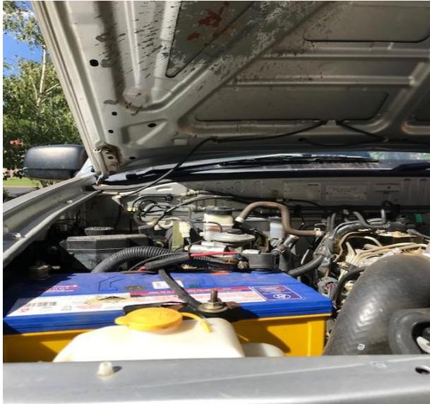
**Photo:** Ute's battery on same side as driver. New sealed battery. Note the damage on underside of bonnet from the previous corroded battery.
